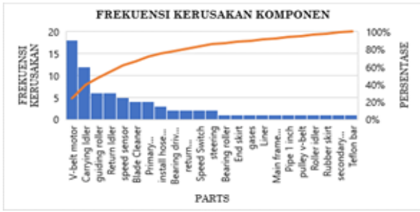
Figure 2. Pareto Diagram of Component 7BA-CNVR-200
